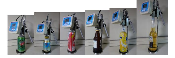
Note 1. Package size that can be measured with this instrument is upto 254mm hight, 80mm diameter. If your sample is over this size, please contact us.
