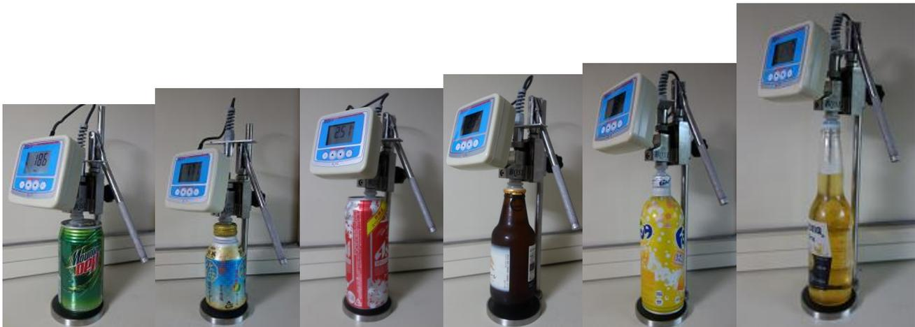
Note 1. Package size that can be measured with this instrument is upto 254mm high, 80mm diameter. If your sample is over this size, please contact us.
