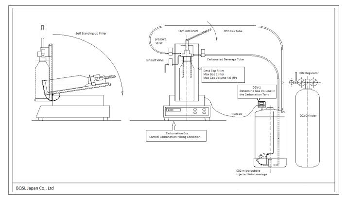
High performance micro bubble carbonator tank is a size of 20 liter. It has a pressure-resist small micro bubble generater at a bottom of the tank. CO2 gas is injected in the beverage to be micro bubbles, and the gas is dissolved in very effectively. High performance micro bubble carbonator tank is equipped with DGV-1 which measures gas volume in real time. When the gas volume reaches the setting value, it alarms you with a buzzer.
