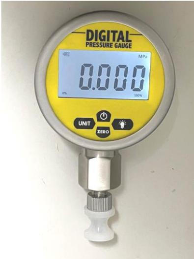
BQSL Vacuum Pressure Tester is a battery type digital pressure tester equipped with semiconductor strain gauge, which was developed to measure vacuum or inner pressure of hot pack beverages/foods. This tester has durably body, high accuracy, and the following features which are difficult with bourdon analogue pressure tester. These features enables you to measure inner pressure more easily and accurately.
